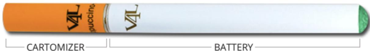
The V4L e-cigarette is made of 2 basic components; a rechargeable battery and a disposable cartridge (cartomizer). The cartomizer screws on to the battery and, when puffed, creates a vapor that simulates the smoking experience. The battery is a lithium-ion rechargeable battery which can be recharged and reused up to 300 times, and powers a heating element inside the cartomizer.
